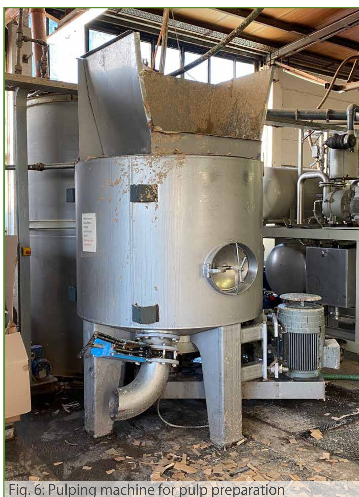
Fig. 6: Pulping machine for pulp preparation
