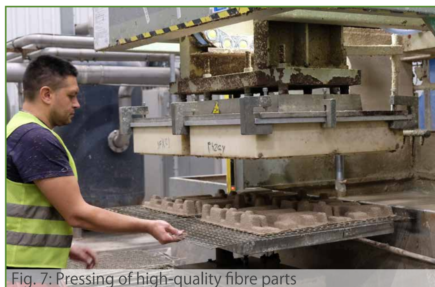
Fig. 7: Pressing of high-quality fibre parts
