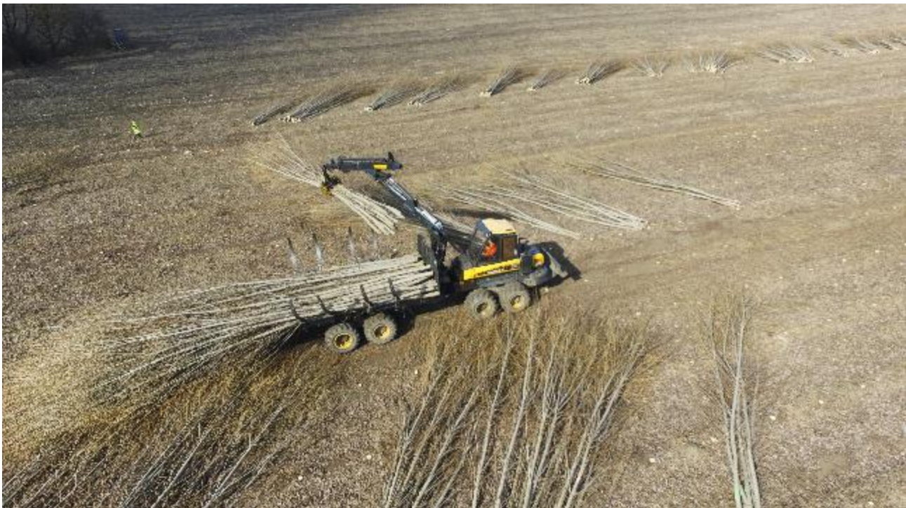
Figure 57 Photo of large forwarder used for on-field transport of prebundled whole trees
