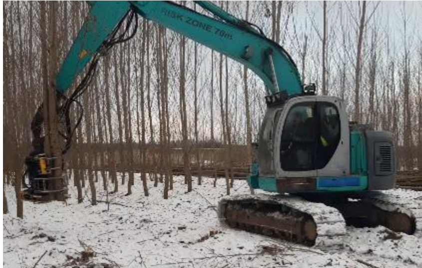
Figure 56 Photo of tracked feller buncher harvester with shears
