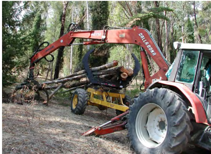
Figure 5. Clambunk skidder attachment for farm-tractor based skidders.
