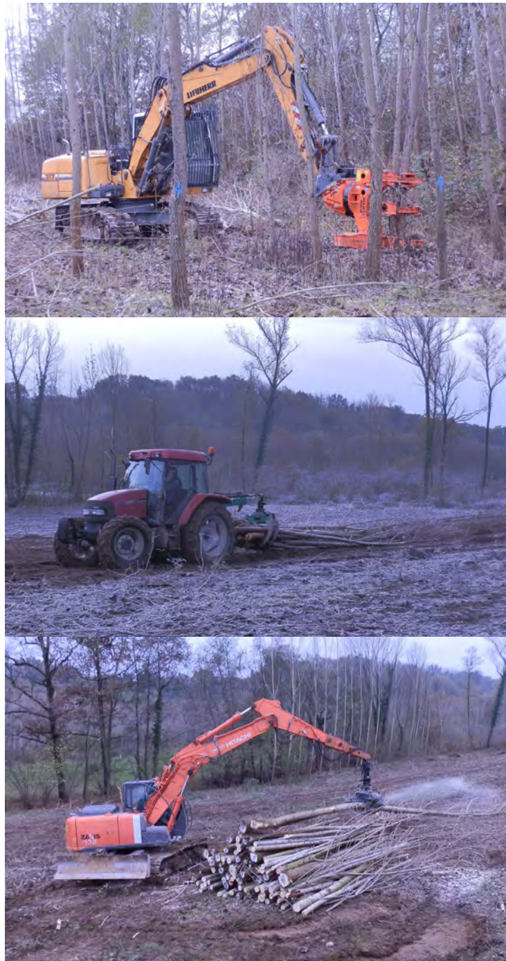
Figure 1. Felling and bunching trees with the excavator-based feller-buncher ( Top ); skidding bunches with the forestry-fitted farm tractor ( Middle ); crosscutting stems into 4-m logs with the excavator-based grapple saw ( Bottom ).
