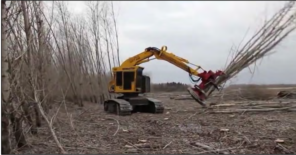
Figure 38 Photo of tracked feller buncher harvester with hot disk harvesting a hybrid poplar plantation in Minnesota, USA.
