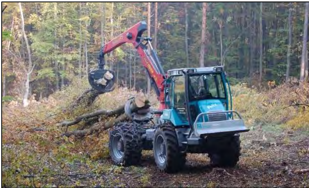
Figure 39 Photo of clambunk forwarder used for on-field transport of prebundled whole trees
